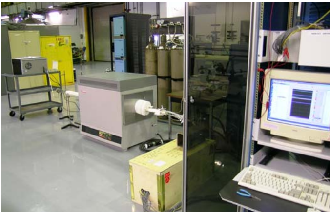
Fig. 7. Long duration 1200 °C thermocouple test setup.
