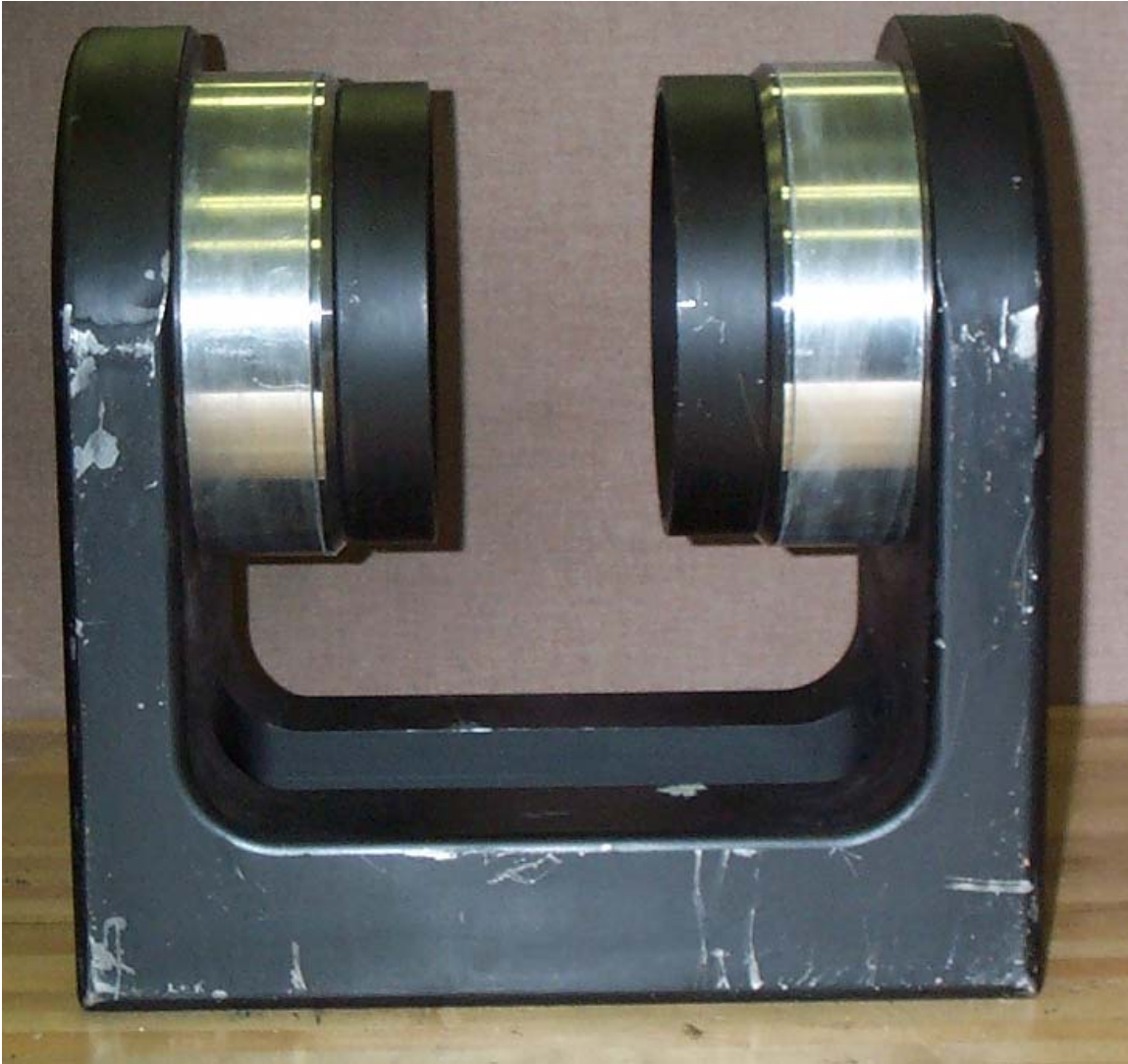
Figure 9. Assembled magnet. The frame is the large “U” shape painted steel (paint marred in the process of assembly). The magnet holders are the large aluminum disks attached to the inside top of the frame. The pole faces are the black steel pieces mounted on the magnet holders.
