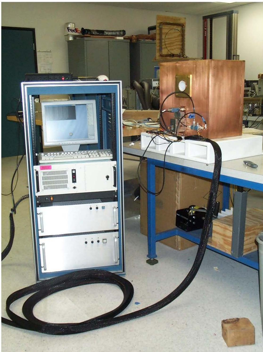
Figure 10. The completed system. The magnet, RF coil and VILNAD are in the enclosure sitting on the table to the right. The components in the rack enclosure from top to bottom are: LCD monitor and keyboard; Industrial PC chassis; Trim coil power supply cabinet; RF power amplifier cabinet. The interconnecting cable assembly is 6 meters long.
