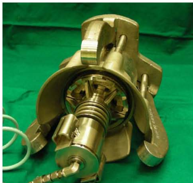
Fig. 8. Installation Tool in Hanford Connector
