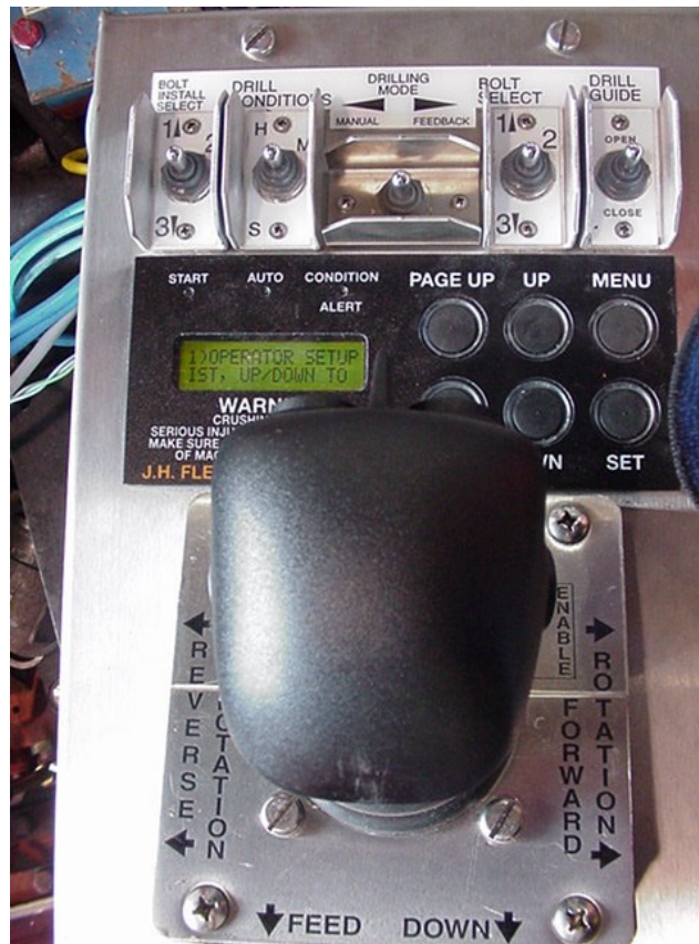
Fig. 1 Drilling Feedback Control System Developed by the J.H. Fletcher & Company
