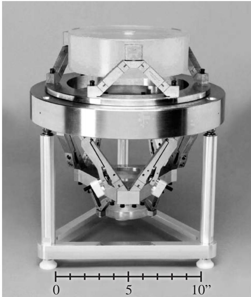
Fig 1. Photo of the MET optical system resting on a stand. Photo courtesy of John Taylor, LLNL.
