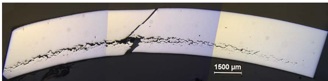
Figure 7: Cross-sectional micrograph of internal crack and pores developed in an unhardened AerMet 100 target impacted at 1.55km/sec shown in Figure 6.
