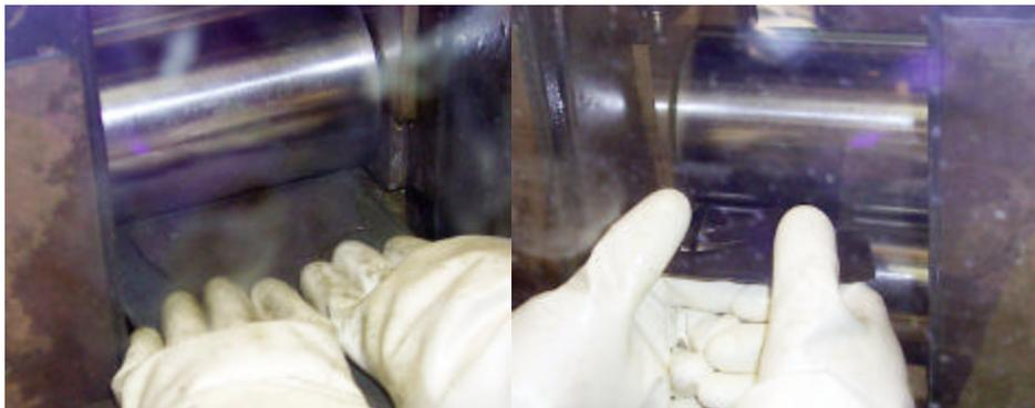
*Figs. 3 and 4. Feeding and catching the disc during the rolling operation.*
