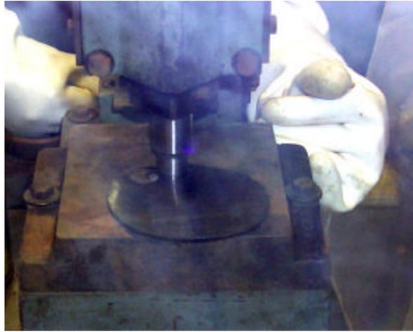
*Fig. 6. Plutonium foil being punched out of the disc with the stamping machine.*
