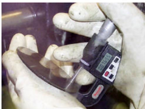
*Fig. 5. Monitor the thickness of the disc during the rolling to decide whether further rolling is necessary.*
