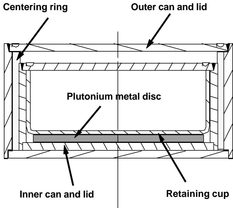
Fig. 8. Schematic drawing of the cans. All the parts, except for the plutonium disc, are made of stainless steel.
