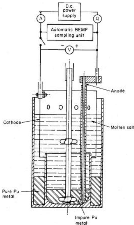
*Fig. 1. Schematic of electrorefining cell showing major features.*
