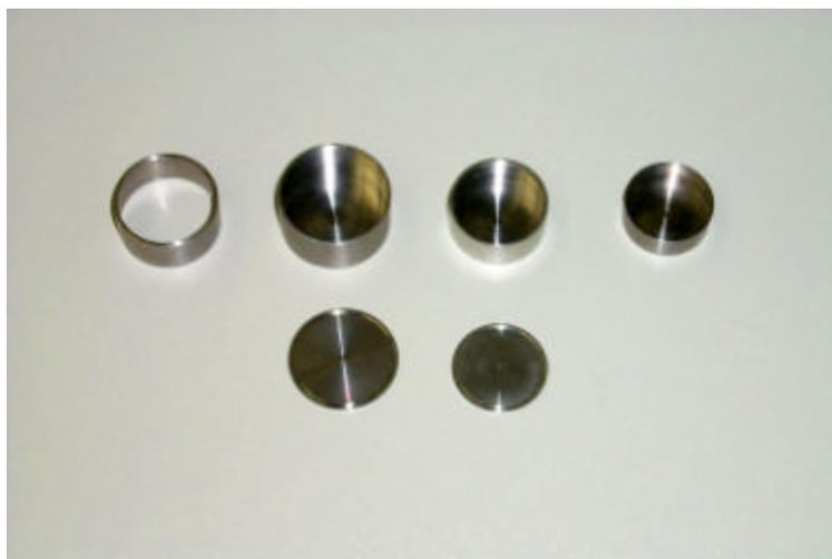
Fig. 9. Picture of stainless steel cans and parts. The right-hand side of the picture shows the inner can, lid, and retaining cup. The left-hand side shows the outer can, lid, and the centering ring.
