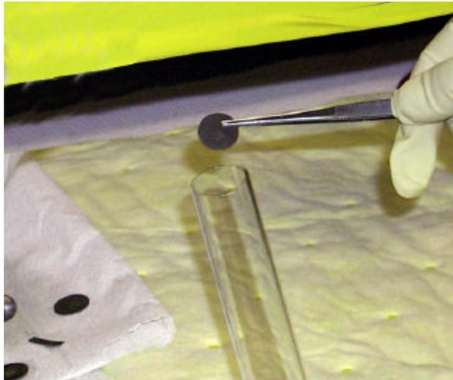
*Fig. 7. Plutonium foils are stored in glass vial to reduce oxidation and contamination. The glass vial is transferred to an inert glove box for encapsulation.*
