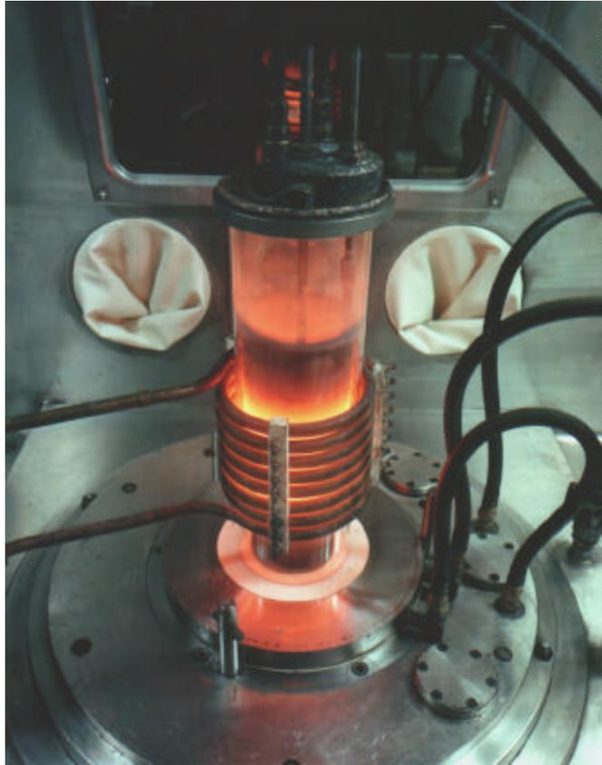
*Fig. 2. Furnace to cast plutonium metal into ingot.*
