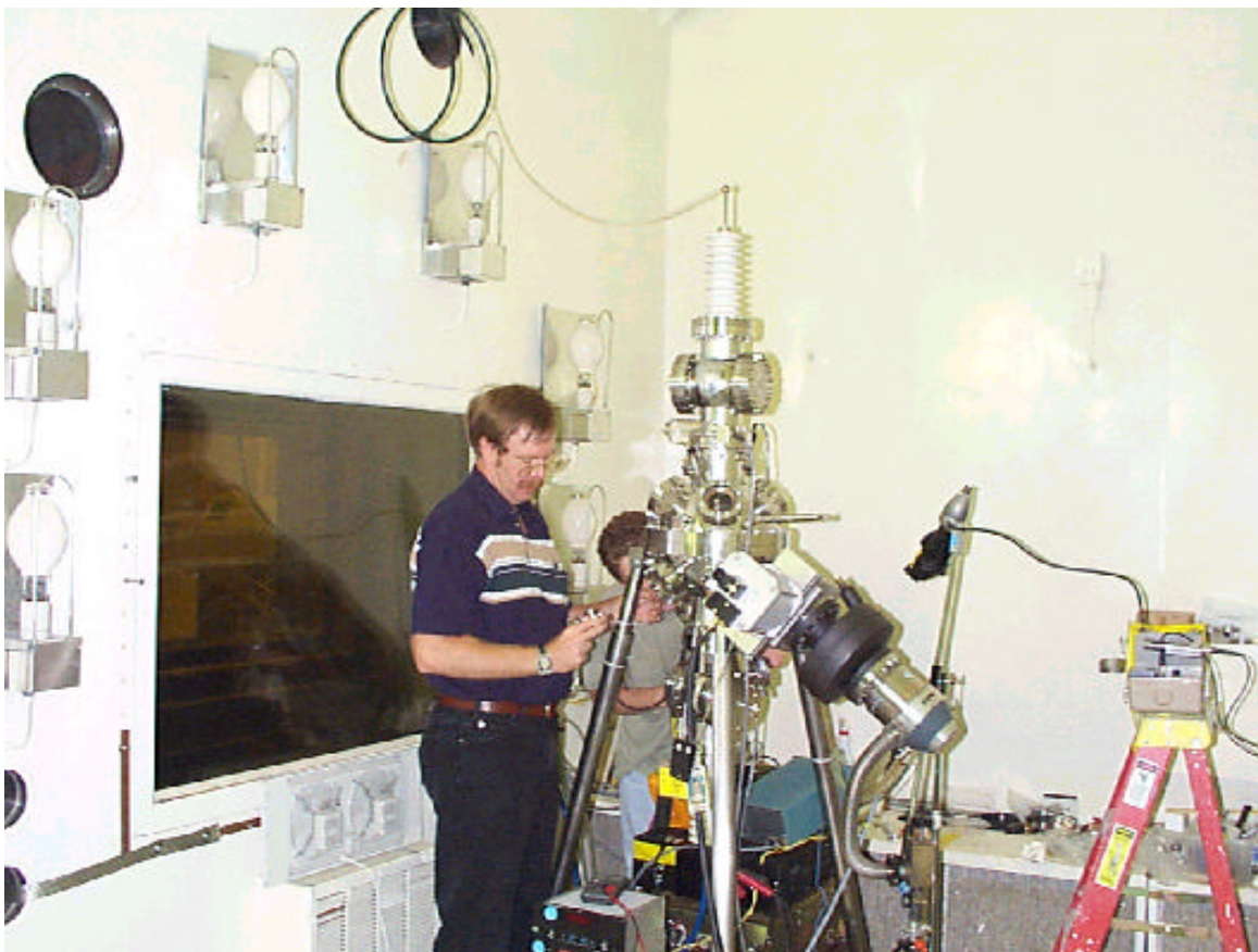
Figure 7. A picture of the entire system in the hot cell. Power supplies are located outside the hot cell.
