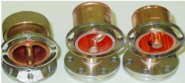
Figure 7: Copper mockups of the HOM couplers. Left is old design, in the middle version -2, right version -4.
