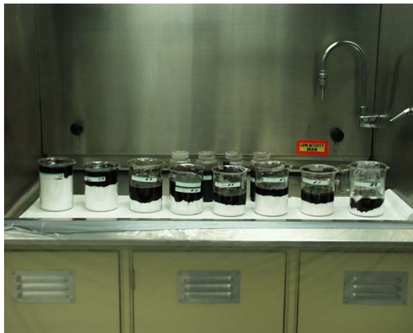
Fig. 2: Photograph of Test Samples During Solidification
