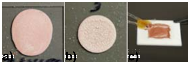
Figure 8. a) Drop-cast thermite on glass using 200 mg/mL solids with 16% FC-2175, and b) 300 mg/mL solids with 20% FC-2175. c) Drop-cast thermite on bare silicon with an alumina housing using 300 mg/mL with 20% FC-2175.
