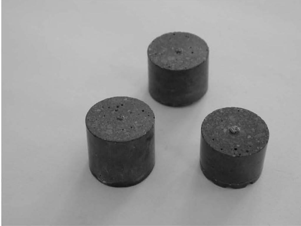
Fig.4 Graphite concrete samples, diameter 21 mm
