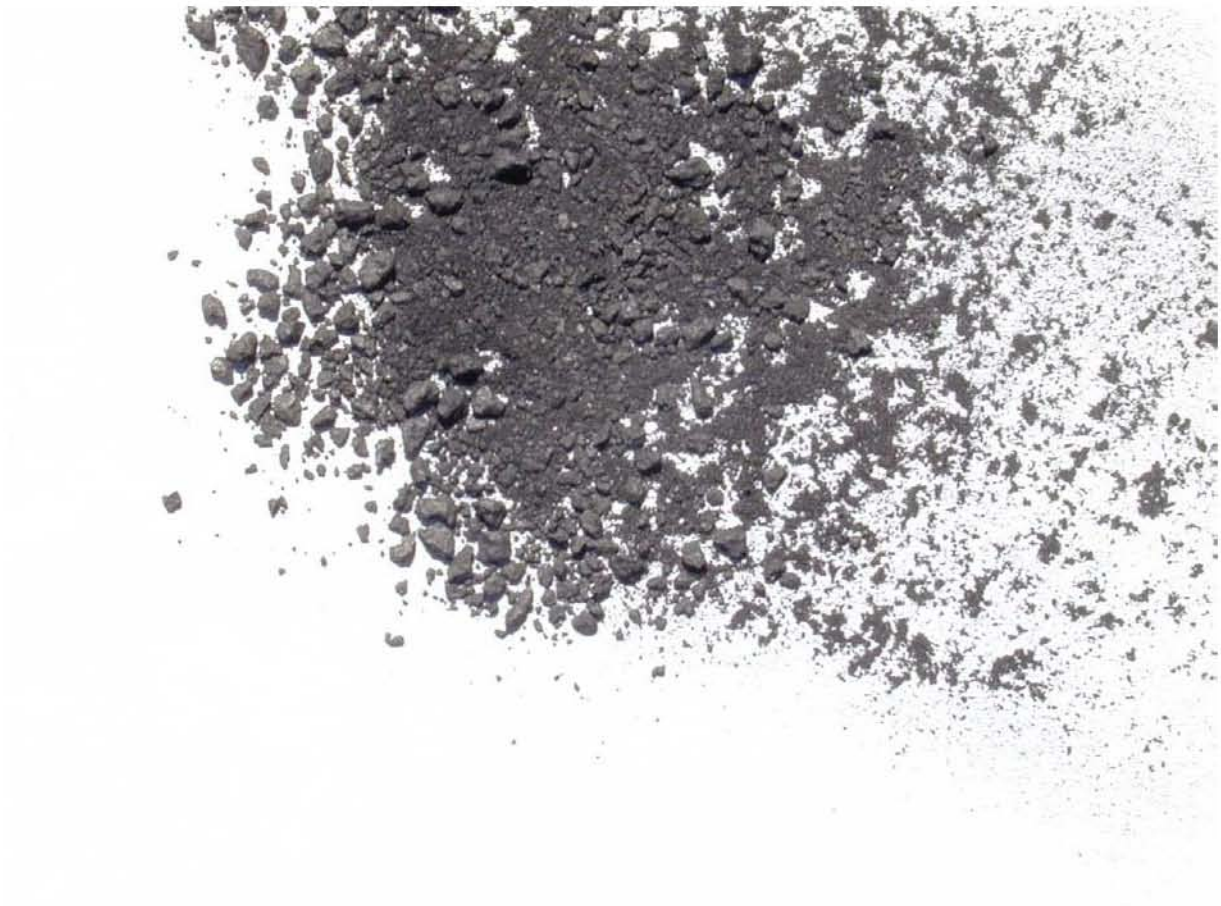
Fig. 3 Crushed graphite, maximum particle size 6 mm
