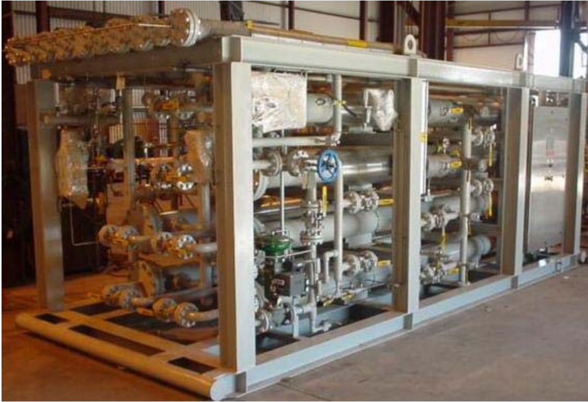
Figure 2. Membrane skid for NTE pilot test.
