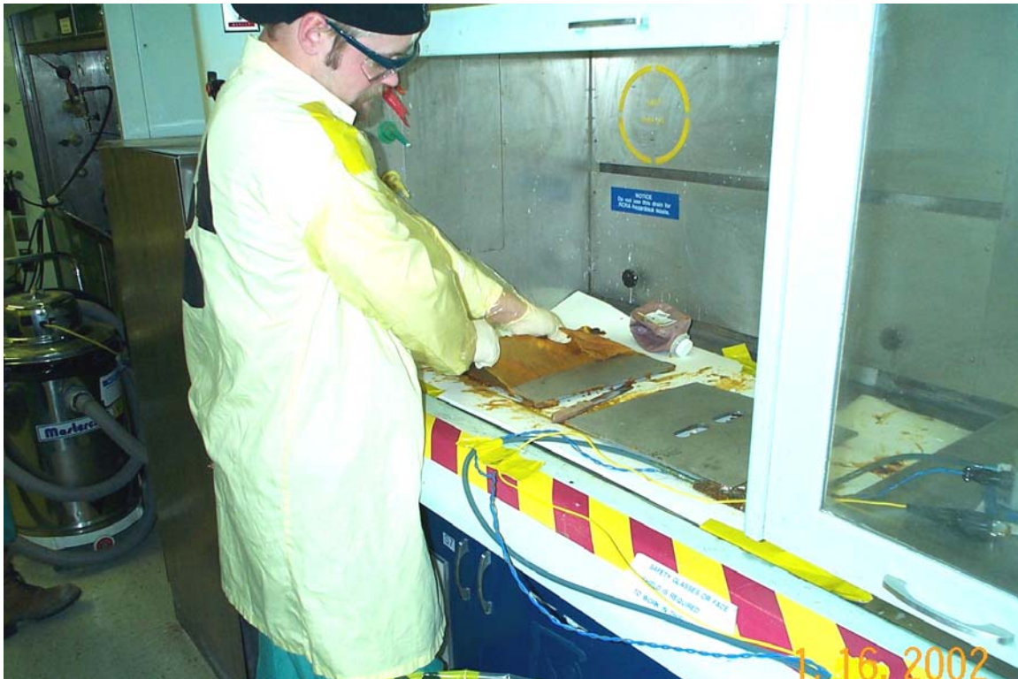
Fig. 3. Electrolyte coating being stripped away from the surface.
