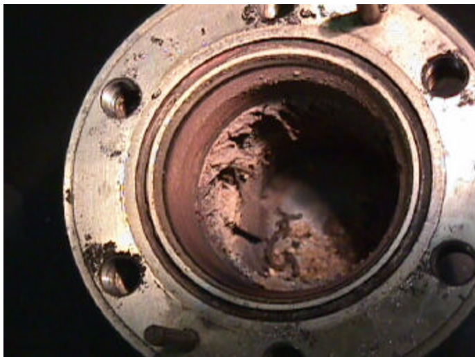
Figure 2: Parr Reactor (solids inside)
