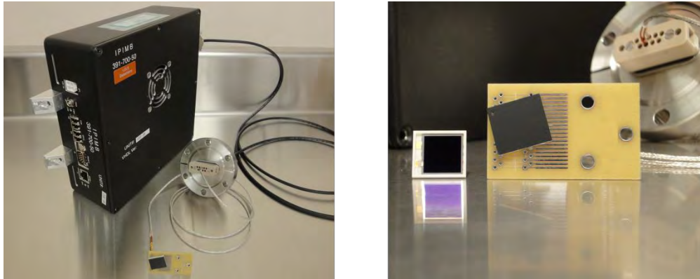
Figure 3. Photograph of the prototype Intensity Monitor with PGP (IMP) to readout photodiodes (left). The photograph on the right side show the commercial x-ray photodiode used for the measurements. A sheet of 30 \mu\text{m} Kapton is glued in front of the diode to block optical light.
