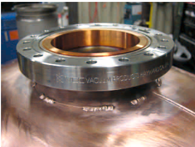
Figure 8. Port repaired by TIG welding.
