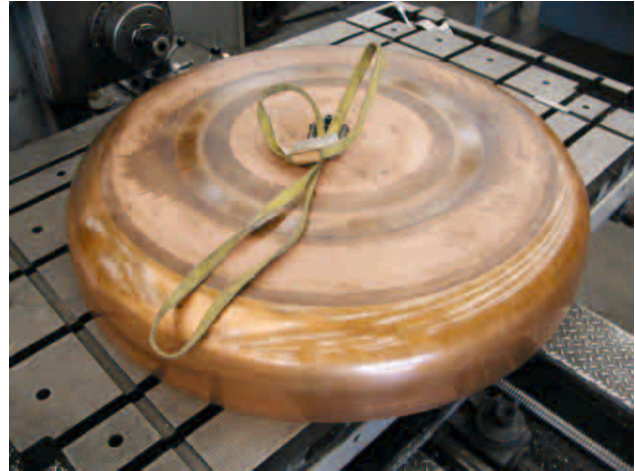
Figure 1: Spun cavity half-shell.
