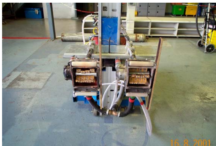
Fig. 4. View of Trelawny Surface Scabbling Unit used in PSA Facility
