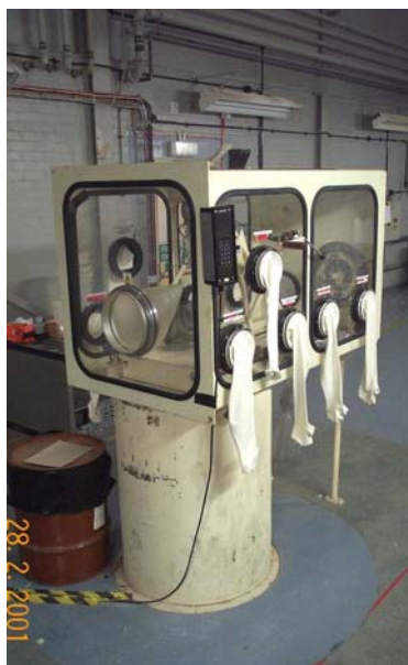
Fig. 3. Glovebox on Roof of NCL used for Tooling Maintenance
