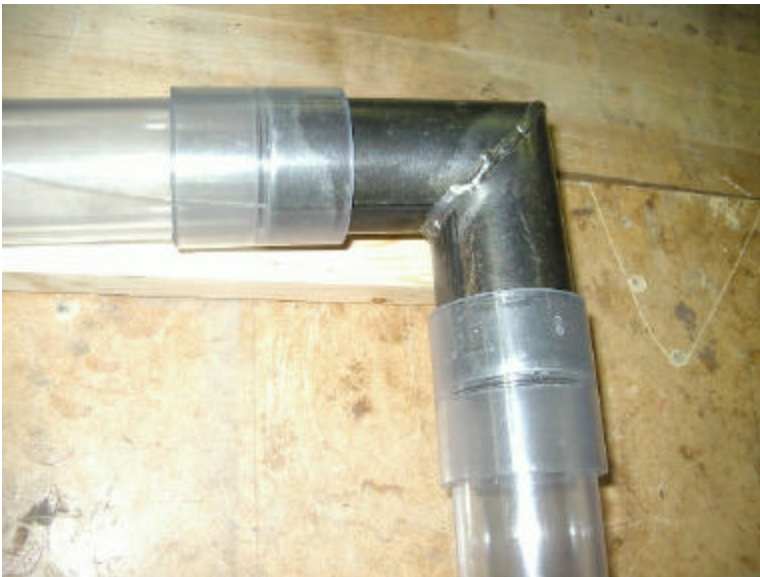
Figure 4. Tether abrasion test in mitered corner
