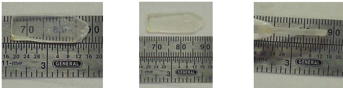
Figure 1. Photographs of a large \text{RbGd}_2\text{Br}_7:\text{Ce} crystal grown at RMD.
