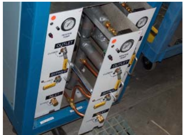
Figure 4: Heater units inserted into a rack. Heater assembly for Cavity 5-2 is shown partially removed to show the polyurethane slide.
