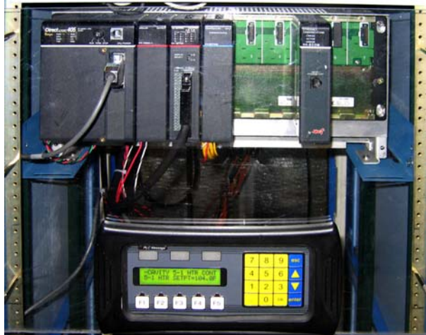
Figure 5: PLC and EZText operator interface panel mounted in the control rack.
