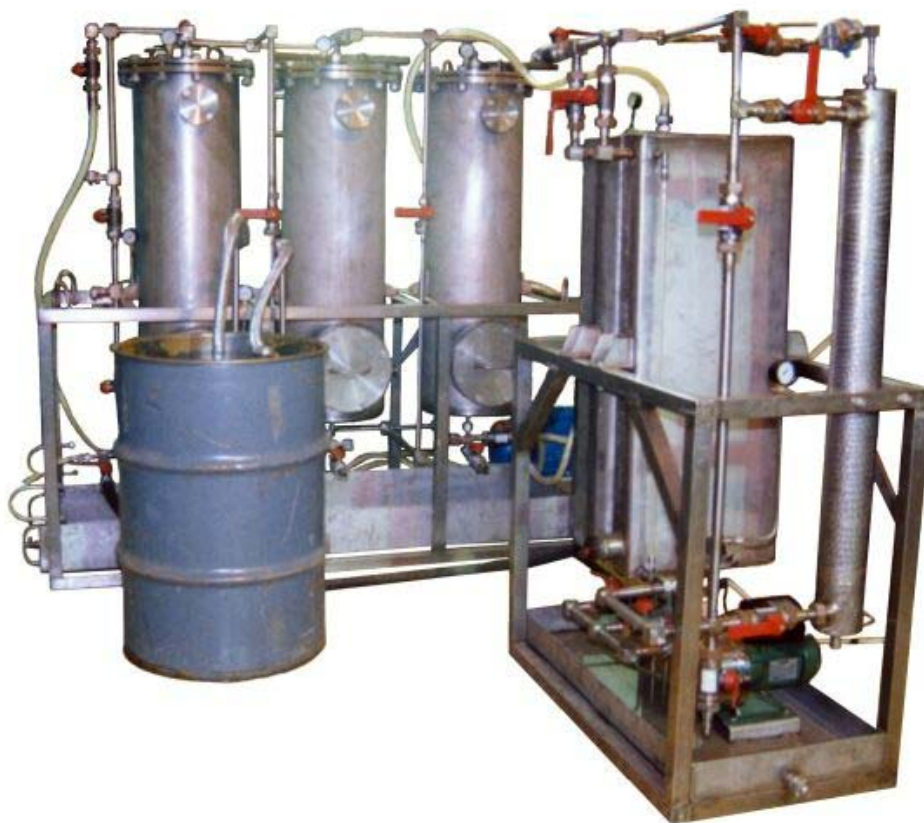
Fig.1. Mobile modular installation "Aqua-Express" for clean-up of LRW.
