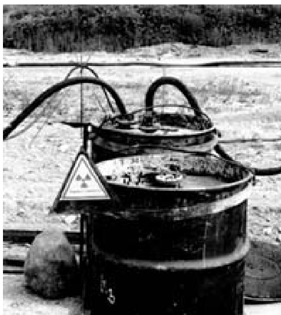
Fig.4. Filter-container with synthetic inorganic sorbent.
