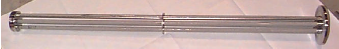
Figure 2. 7-tube bundle and each tube had: 9.5-mm i.d., 12.7-mm o.d., 1.01-meter long.
