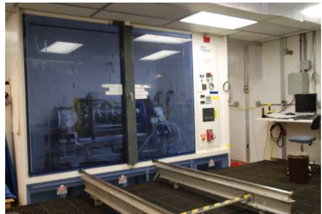
Figure 1: EP facility with an ILC 9-cell cavity installed in the main EP cabinet.
