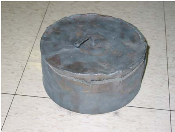
Figure 1. H13 only disc can with a big crack
