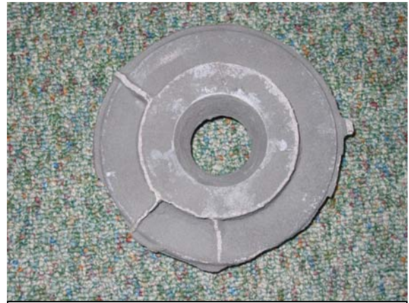
Figure 4. H13 only disc, front, note 'ribs' where the sand mold cracked
