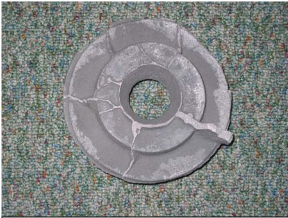
Figure 3. H13 only disc, back, note 'ribs' where the sand mold cracked
