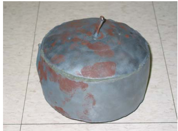
Figure 2. Blown H13/WC disc can
