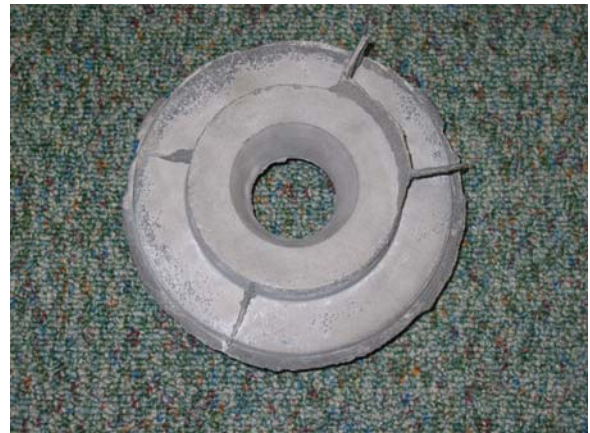
Figure 6. H13/WC disc, back, note 'ribs' where the sand mold cracked
