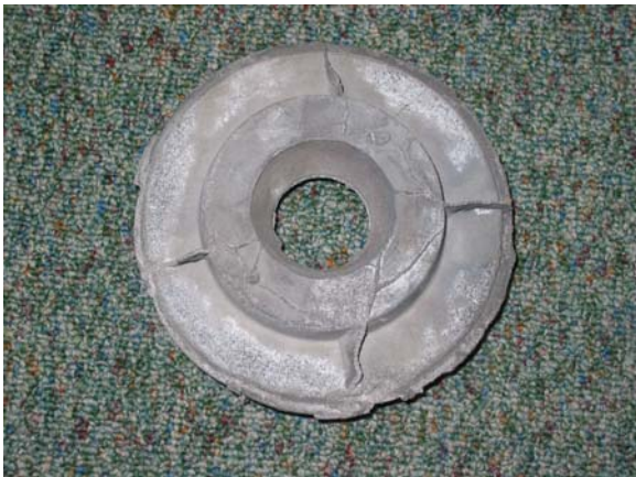
Figure 5. H13/WC disc, front, note 'ribs' where the sand mold cracked
