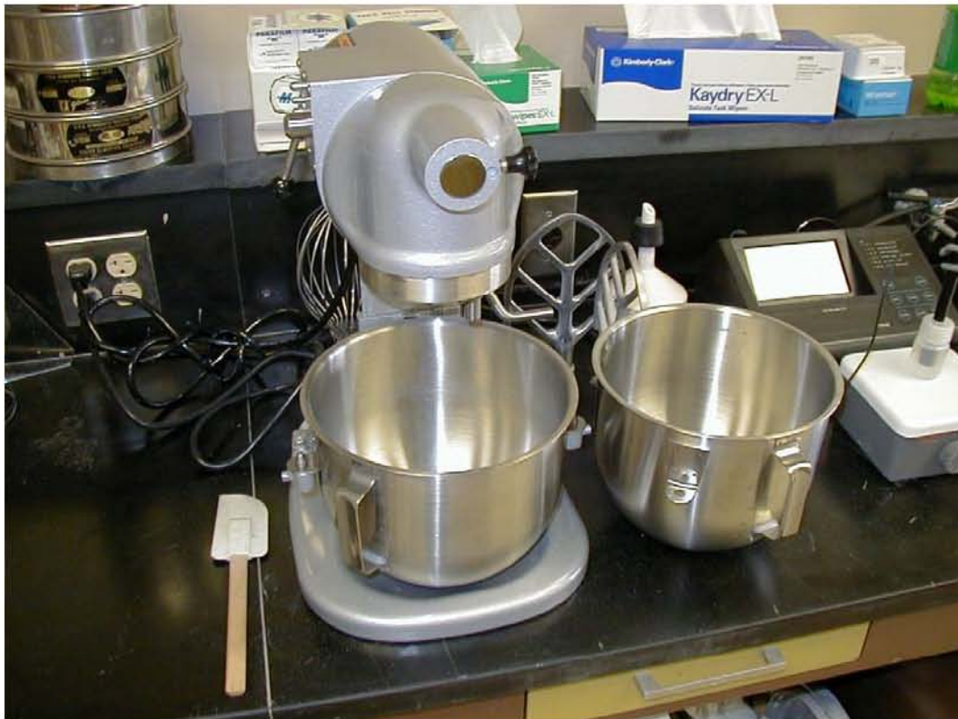
Figure 1. Laboratory mixer used to prepare mortar.
