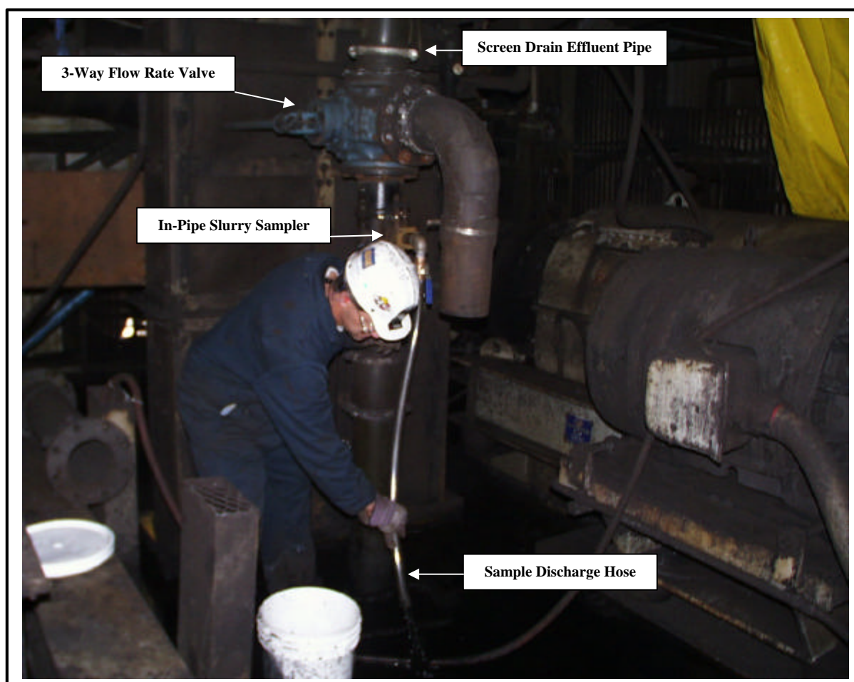
An in-pipe sampler was used to collect the screen drain sample from the screen bowl centrifuge
