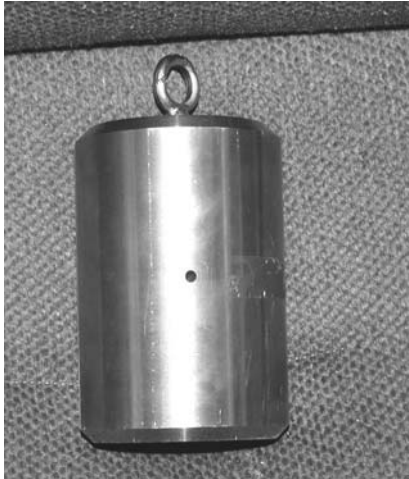
Figure 2, “Boat Anchor” Shield, Showing 0.200 inch Collimator Aperture
