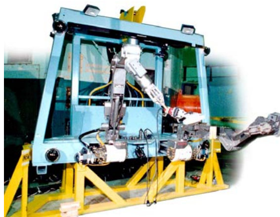
Fig 4. An innovative control system will enable the Dual Arm Work Platform to complete D&D activities more quickly with increased accuracy.
