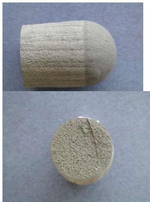
Figures 3 – 6: Confinement burnout, Test 1. Insert was embedded in a clay crucible filled with silica sand. The confinement came from the weight of top sand. The heating rate was 0.5°C/min from room temperature to 500°C, followed by a sintering to 1100°C for two hours.
