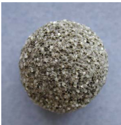
Figures 7 – 9: Confinement burnout, Test 2. Insert was embedded in a metal container fully filled with silica sand and covered by a metal lid. The confinement was introduced by the metal container's resistance to expansion. The heating rate was 0.5°C/min from room temperature to 500°C, followed by a sintering to 1100°C for two hours.
