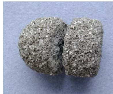
Figures 7 – 9: Confinement burnout, Test 2. Insert was embedded in a metal container fully filled with silica sand and covered by a metal lid. The confinement was introduced by the metal container's resistance to expansion. The heating rate was 0.5°C/min from room temperature to 500°C, followed by a sintering to 1100°C for two hours.
