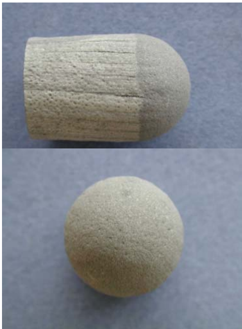
Figures 3 – 6: Confinement burnout, Test 1. Insert was embedded in a clay crucible filled with silica sand. The confinement came from the weight of top sand. The heating rate was 0.5°C/min from room temperature to 500°C, followed by a sintering to 1100°C for two hours.
