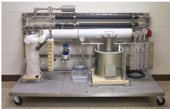
Figure 4. Pyrolysis process with catalytic conversion
