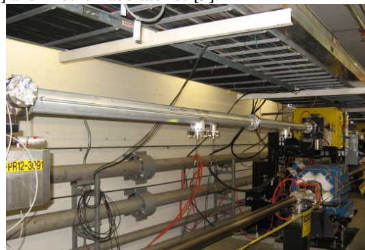
Figure 2. Layout of the installation in PEP-II LER: Groove chambers (left chamber on upper beam line) and smooth chamber (right).
