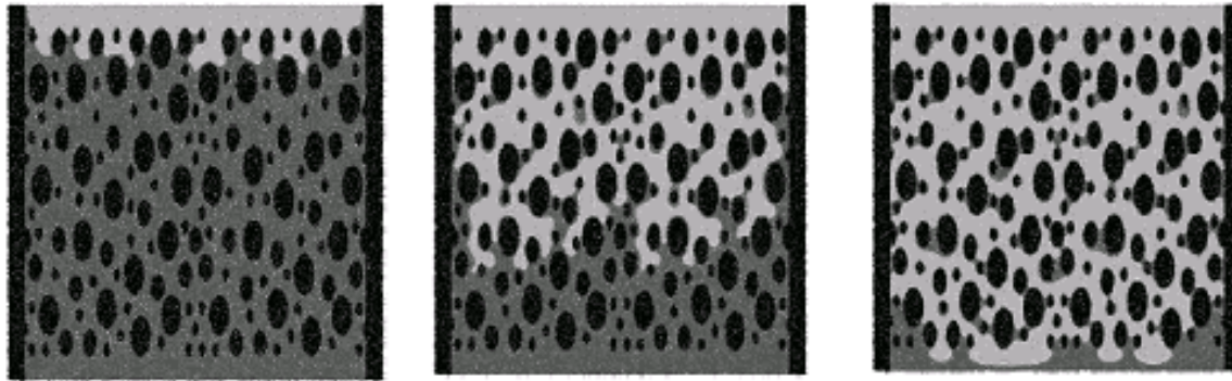
Figure 2: Three stages in a 2-dimensional simulation of the gravity driven penetration of a dense non-wetting fluid into an anisotropic porous medium
