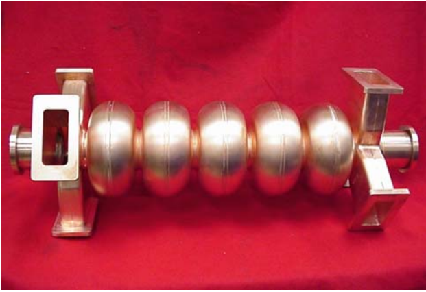
Figure 2. Copper five-cell model of the high-current cavity with waveguide end groups.
