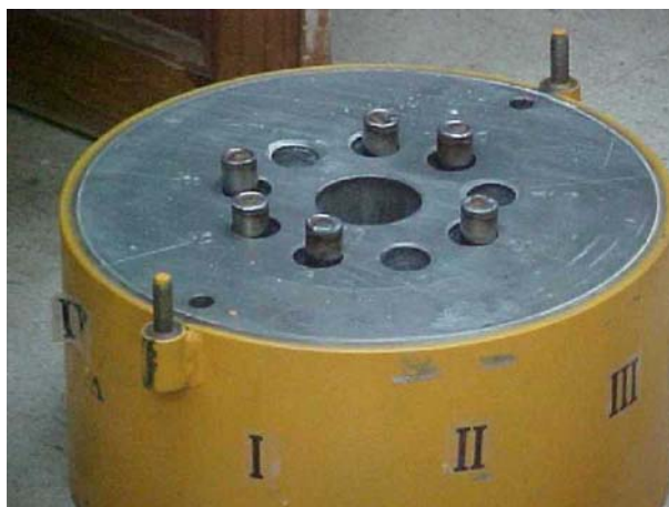
Figure 3. Lead shield and stainless steel capsules.
