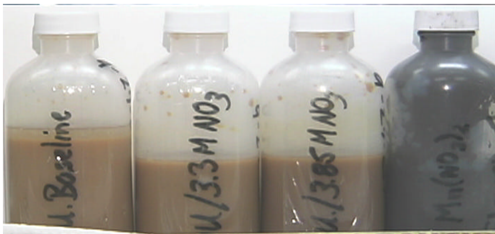
Figure 2. The four simulant slurries; baseline, 3.3 M nitrate, 3.85 M nitrate, manganese
