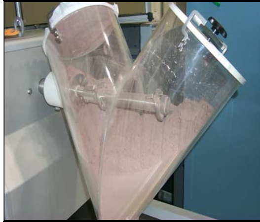
Figure 4: Rotary V-Blender
