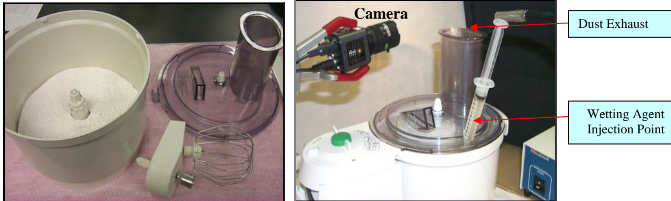
Figure 3: Bench Scale Assembly at SRNL
