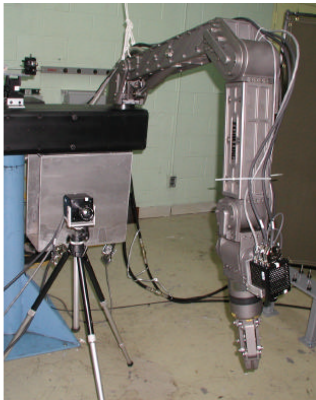
Figure 1: Experimental testbed including a Schilling Titan II hydraulic manipulator with a fixed camera and an in-hand camera
