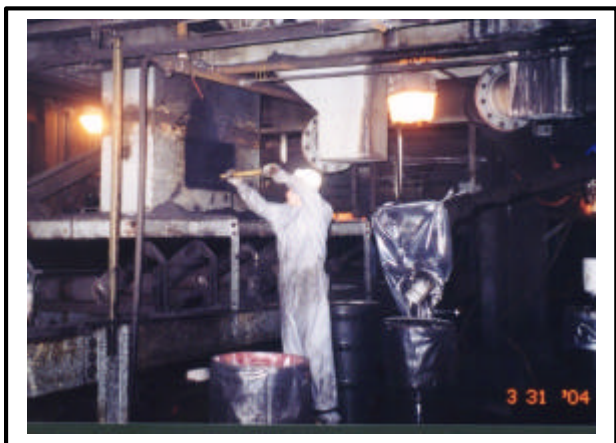
Sampling Screen Bowl Centrifuge Filter Cake
