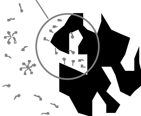
Figure ii. Surfactant adsorption on porous unburned carbon.
