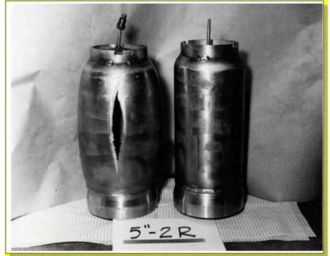
FIG 3. PCV (INVERTED) AFTER AND BEFORE THE BURST TEST
