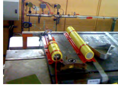
Figure 3: Test BLMs installed on top of the main magnet. The detectors are installed according to Fig. 2.
