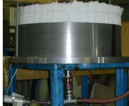
material in a filled CFRP mould of full scale. The tests will give us information regarding flow of resin/leveling in the mould, adhesion of resin to the membranes and canister and most important possible formation of cracks due to exothermic reaction/thermal expansion.
