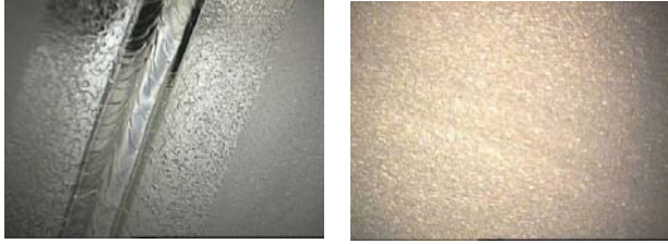
Figure 3: Picture of the inner surface of the equatorial weld before (left) and after (right) removing 60 µm by centrifugal barrel polishing (Courtesy of T. Saeki).
