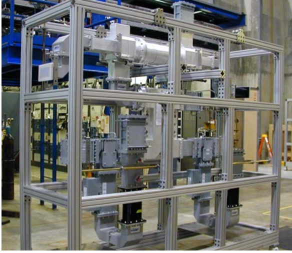
Figure 2: A two-feed sub-unit of the power distribution system in its support frame. When installed, the front wall of the frame will be removed, and the U-bends reversed to go under the remaining wall.
