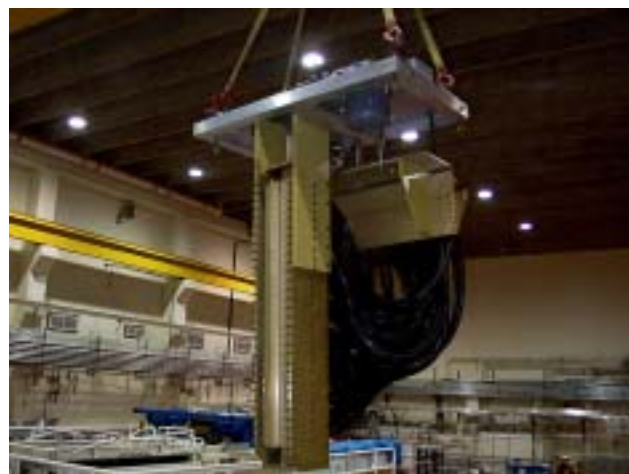
Figure 3 Cable header and load protection switch assembly
