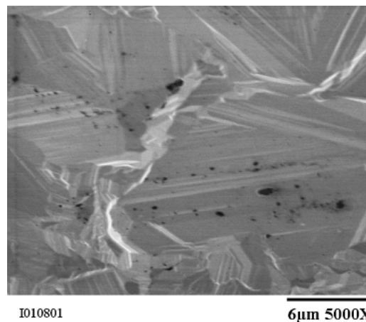
Fig 3. Poly-Si layer grown at 950^\circ\text{C}
