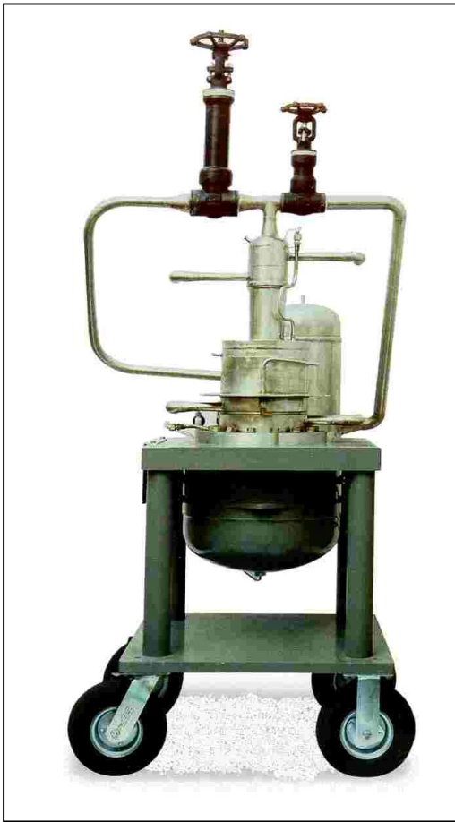
Figure 5. An early prototype linear compressor driven OPTR
