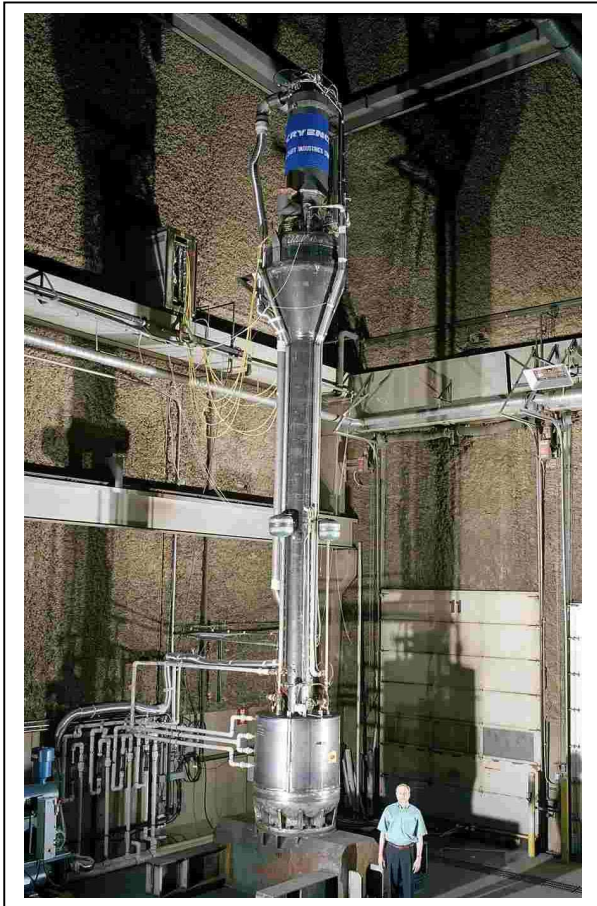
Figure 2. The 500 gpd TASHE-OPTR. The natural gas burner is at the very top. The TASHE is the large bulge below the burner and the OPTRs (not visible) are inside the vacuum jacket hear the bottom.
