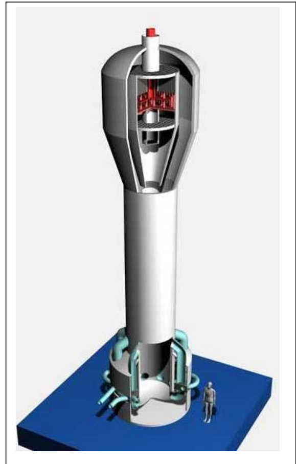
Figure 3. Conceptual configuration, 10,000 gpd TASHE-OPTR
