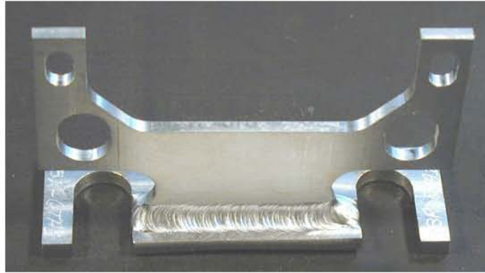
Fig. 1. Baffle support brackets made with a V-4Cr-4Ti alloy for the DIII-D upper radiative divertor
