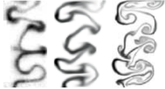
Figure 6. \text{SF}_6 volume fraction at 400 \mu\text{s} for the experimental image (left) the dynamic Smagorinsky Cuervo result (center), the second-order standard MUSCL-type scheme (right).
